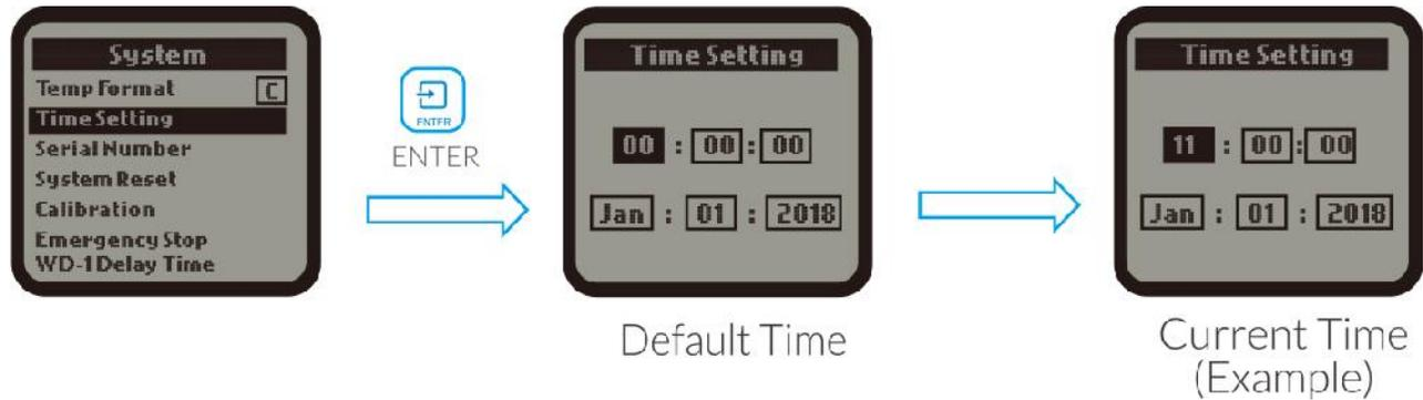
Press ENTER button and the HOUR will be highlighted and blinking, Press UP or DOWN button to change the hour. Press ENTER button again and the cursor will skip to the next, the MINUTE will be highlighted and blinking. Similarly, you can change the MINUTE and SECOND. When the 1st line of time ( HOUR:MINUTE:SECOND) has been changed, press ENTER button and the LCD screen will display " Setting saved"
