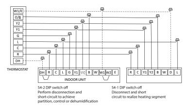
• Wiring for 1H and 1C thermostat
