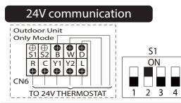
24V must never be connected to S1 – S2. All wiring must be in compliance with the above scenarios. Incorrect wiring will cause irreversible damage to control.
