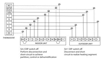
• Wiring for 3H and 2C thermostat
