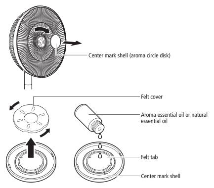
3. Install the felt cover, and put the aroma circle disk back into place. When installing the felt cover, place it in the center mark shell and turn to right. Then put the center mark shell back on the front grille and turn to right.
