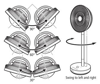
The swing angle can be manually adjusted by 70° upwards, 10° downwards and 60° horizontally.
