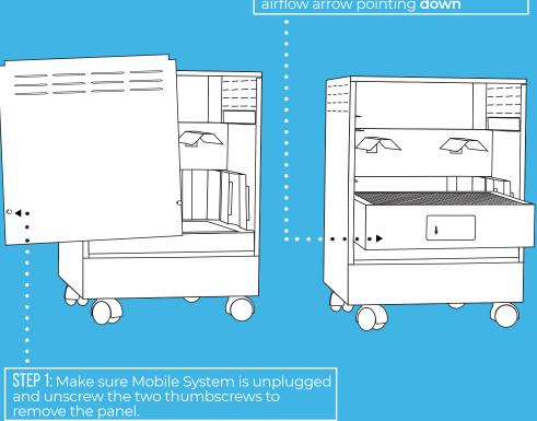
STEP 2: Slide in larger HEPA Filter with airflow arrow pointing down
