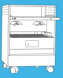
STEP 4: Slide in **smaller Enviroklenz® Air** Cartridge above the UVC lights on the rails with airflow arrow facing **down**
