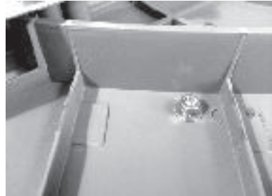
View from the bottom, washer and nut holding the bolt of the attachment and stopper
