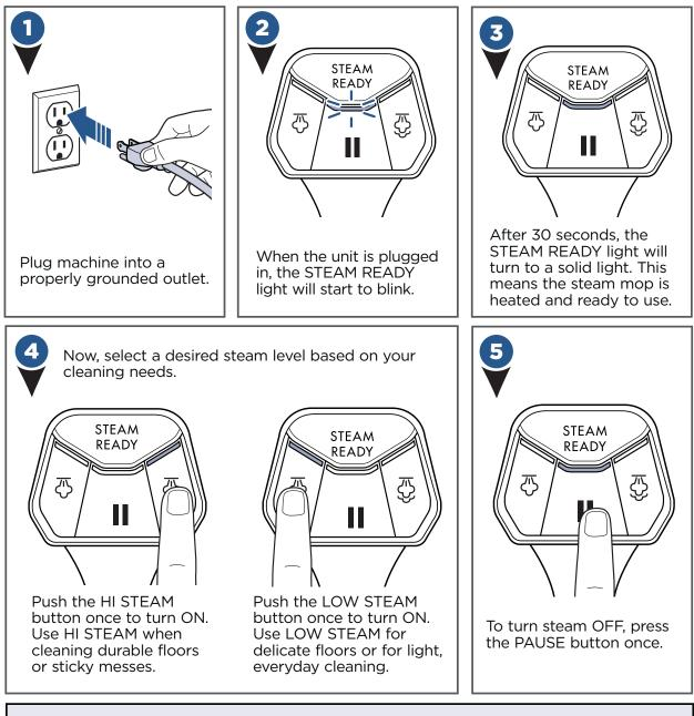
**NOTE:** You must wait until the STEAM READY light is a solid color before selecting your desired steam level. Upon the first use of your steam mop or first use after refilling the water tank, the pump may make a "knocking" sound. This is normal and will diminish after a few seconds.
