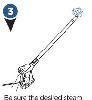
Be sure the desired steam setting is selected, then push the trigger located under the handle of the Handheld Pod to release steam.
