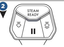
Make sure the STEAM READY light is solid before selecting the appropriate steam level based on your hard floor cleaning needs.
