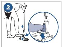
To clean above floors using the **Extension Wand**, step down on the pedal located on the back of the steam mop and lift up to release the Extension Wand.
