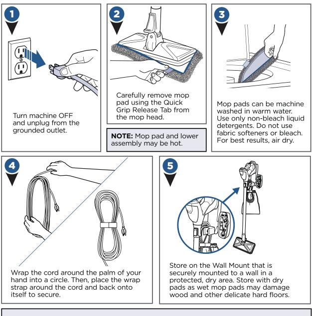
**NOTE:** Unit does not stand up on its own. If you are not using the Wall Mount, make sure your steam mop is stored in a safe place, in the upright position against a firm surface to prevent from falling over.
